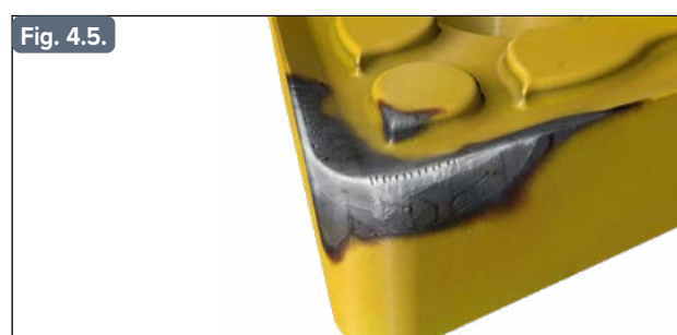
Chipping of the cutting edge
