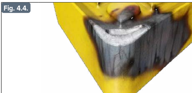
Face wear in the form of crater wear
