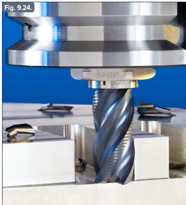
FINISHRED "two-in-one" endmill
