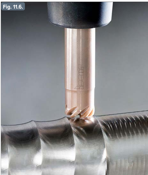
Fig. 11.6. Solid endmill from ceramic cutting material
