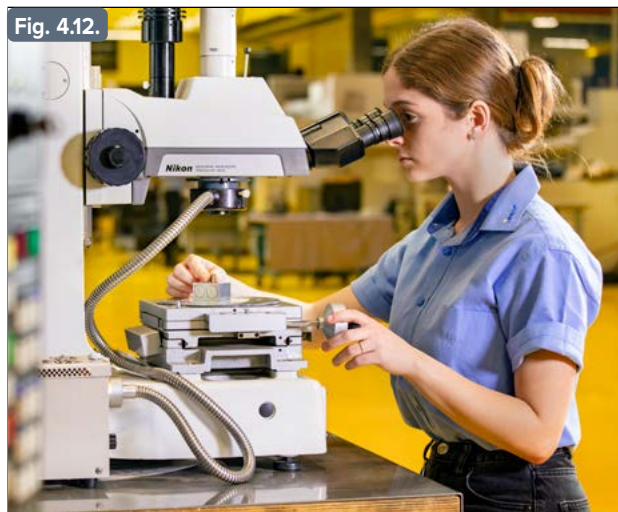
Checking tool wear by use of computerized microscope in ISCAR's Technical Center
