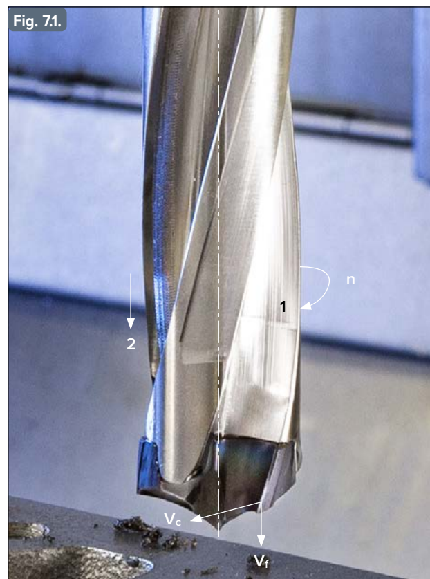
Fig. 7.1. Motions and motion velocities in drilling.
