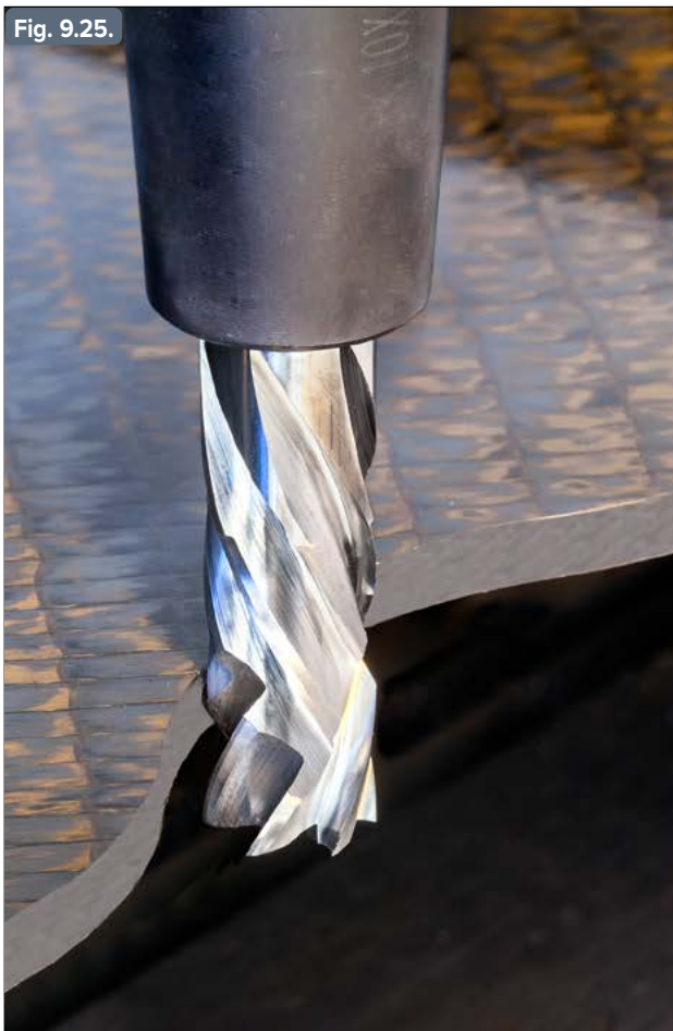
Fig. 9.25. Solid carbide endmill with right- and left-hand helix for machining composite materials
