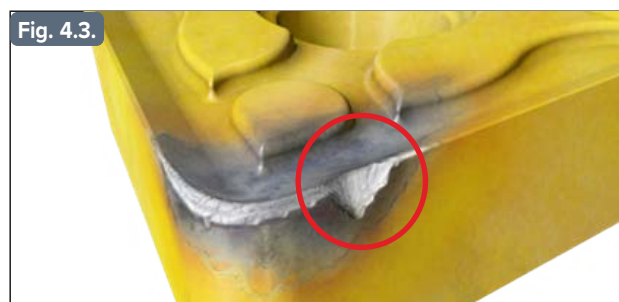
Local flank (notch) wear
