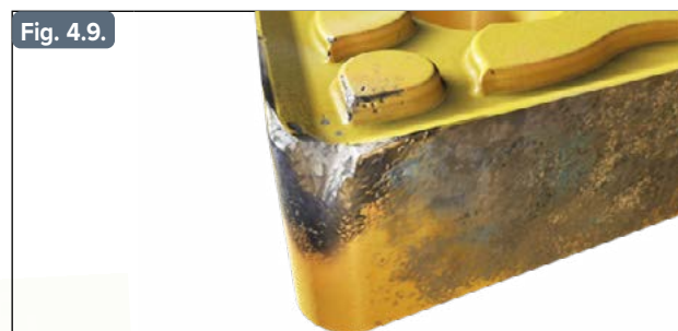
Catastrophic failure (fracture) of cutting edge
