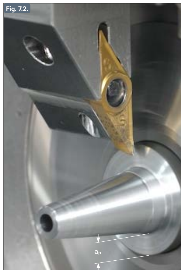
Depth of cut in turning
