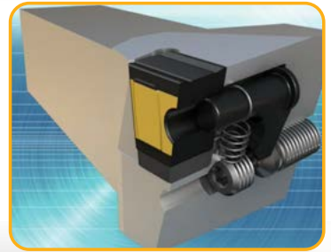
Lever Lock Accessible from Both Tool Sides
